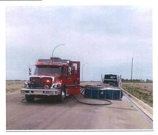
An annual pump test of the Fire apparatus was performed in May. This is an essential preventative maintenance program that assists in determining the status of the pump in terms of efficiency and potential wear. The service provider also performs an apparatus inspection and pump service.
