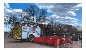
DFR supporting Langham FD with personnel, water shuttle, and relay pumping to LFD apparatus
