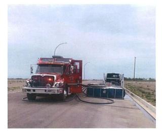
An annual pump test of the Fire apparatus was performed in May. This is an essential preventative maintenance program that assists in determining the status of the pump in terms of efficiency and potential wear. The service provider also performs an apparatus inspection and pump service.
